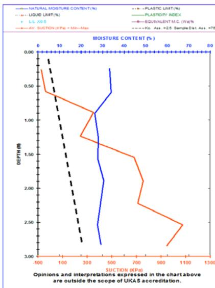
Although there are high suctions, further investigations revealed there was no evidence of root induced desiccation. The high suctions were a product of either the soil mineralogy, or a problem with the Whatman’s 42 filter paper - this has been explored in previous editions and is a well-recognised issue in our industry.
