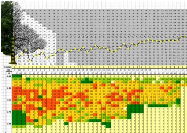
Above, the Disorder Model delivers an estimate of ground movement of around 40mm, taking into account species, climate and soil type.
