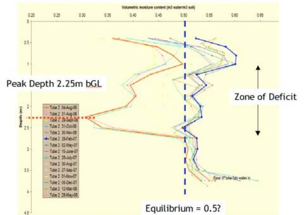
Above are the general characteristics of the profiles. This is the plot of NP 2 (just outside the canopy and nearest to the 'drip line') which shows the widest seasonal fluctuations with the soil rehydrating completely, recovering in one season.
