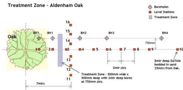
Comparing ground movement with readings over the last few years we hope to be able to determine whether the treatment has delivered a material benefit. The objective is to reduce movement to a level where the tensile resistance of an average building can cope, without cracks appearing - around 15 - 20mm.
