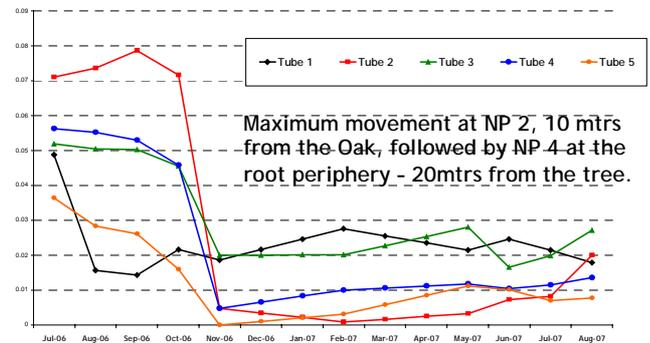
Tim Freeman kindly provided a method of estimating water uptake based on volumetric measure. By multiplying the soil/root volume by the change in volumetric moisture we can estimate the water uptake. Our average 7.3% moisture deficit in  $\pi \times 25^2 \times 1.2m$  average volume of soil =  $0.073 \times 2,355m^3 = 172 m^3 - 172,000$  ltrs in a year.
