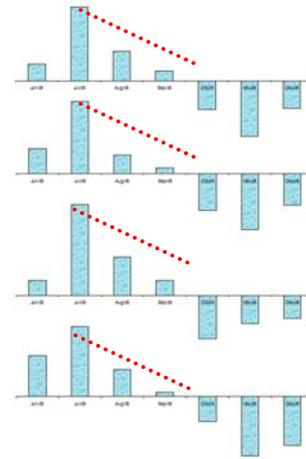
Comparison 'By Month' Ground Movement Profiles from Various Stations across the Willow Footprint Showing the Consistent Pattern in a Dry Year - 2006.
